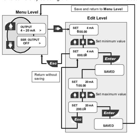
F9.00.L will allow any value from 0.0000 to 99999 and the beginning of the measuring range can be larger than the end of it (inverted output signal). if the back light is ON it is not possible to set the current loop.
