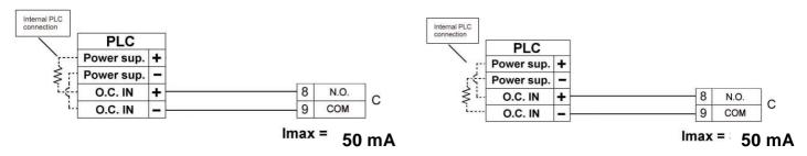
Connection to a PLC / Instrument digital input with separate Power Supply
