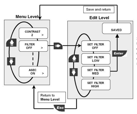
Select the averaging level to dampen LCD indication, output and relay response. **OFF:** no dampening effect, near instantaneous response.
