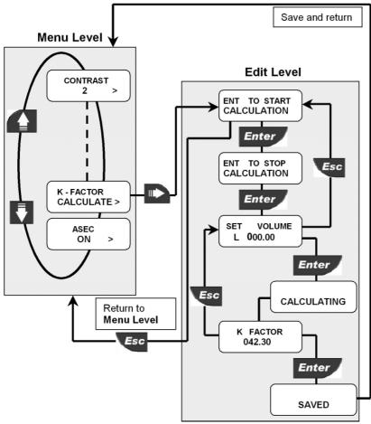
Press ENTER to start calculation. Switch on a pump or open a valve. F9.00.L starts counting pulses from the sensor.
