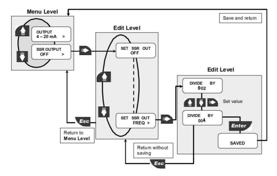
In FREQUENCY mode the SSR output will simulate the sensor frequency divided by the set value. Enter any value between 002 and 255.
