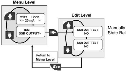
Manually toggle the status of the Solid State Relay (OPT) output for testing
