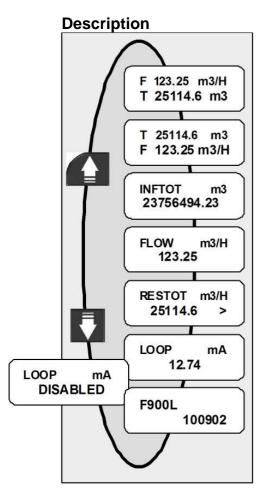
Flow rate and resettable totalizer value
