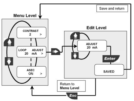
Increment output current value by pressing UP arrow key or decrement it by pressing DOWN arrow key.
