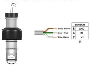
F3.00.H IP65 flow sensor connection
