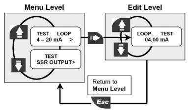
Manually simulate any output current value to test current loop, if the back light is ON the current Loop is disabled.
