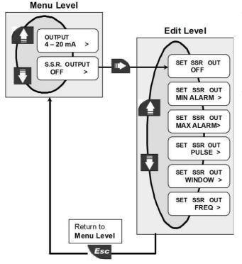
The mode of operation for the Solid State Relay Output (OPT) can be selected between different options: MIN alarm, MAX alarm, volumetric Pulse or Frequency.
