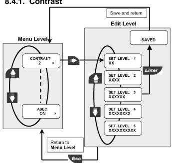
Adjust the LCD contrast for best viewing. Five different levels are available, from 1 for low contrast up to 5 for high contrast.
