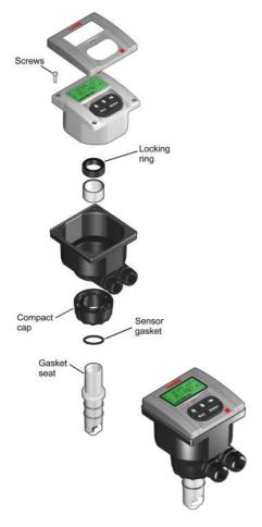
The compact mounting kit F9.KC1 includes the compact plastic adapter with gasket for IP65 watertight installation, the sensor gasket, the compact cap, the locking ring and four fixing screws.
