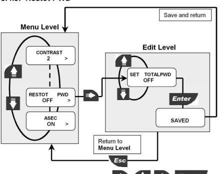
Set ON the Restot PWD to resettable protect the undesired totalizer from reset operations.
