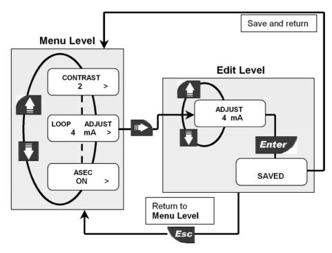
Increment output current value by pressing UP arrow key or decrement it by pressing DOWN arrow key.
