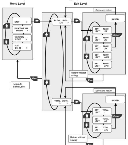
The instrument will automatically convert the values of the two totalizers in the new engineering units.
